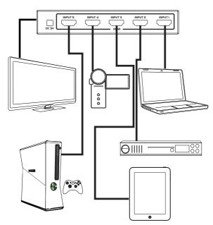
3.Once you have connected all the required source devices and to the HD display, you can connect the power adapter to the proSwitch.H5 and to the electricity
