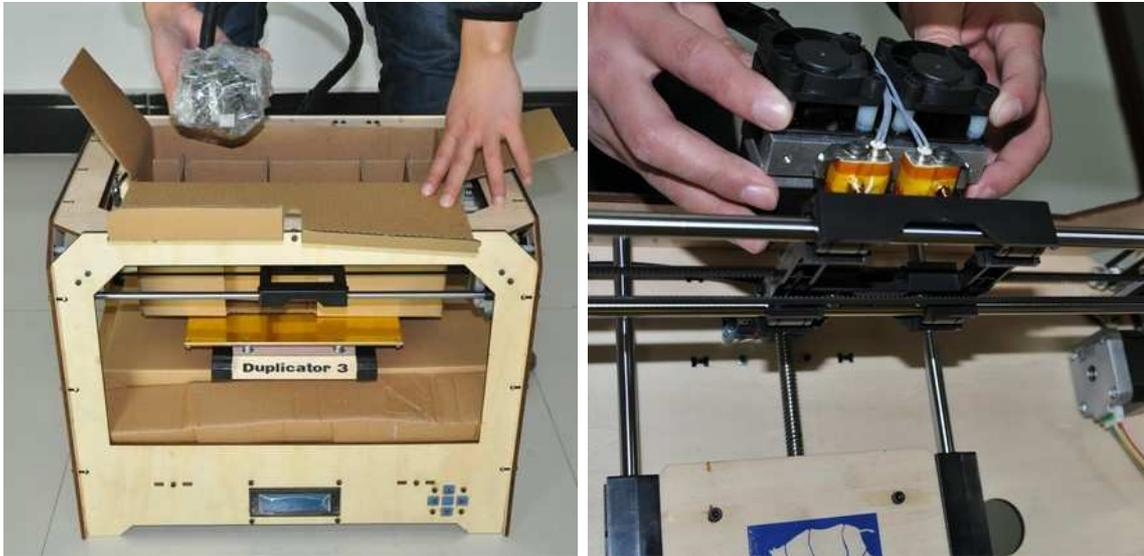
Now you can clear away the cardboard inserts and remove the **Accessory Box** from The Duplicator 3. Be careful of the black plastic **Step extruder MK8+ Mount**.
